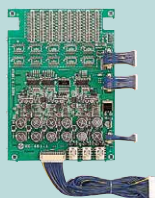
NHR-30K 30-call add-on trunk card • UL listed: UL 1069
