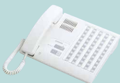
NHX-50M 50-call master station • UL listed: UL 1069
