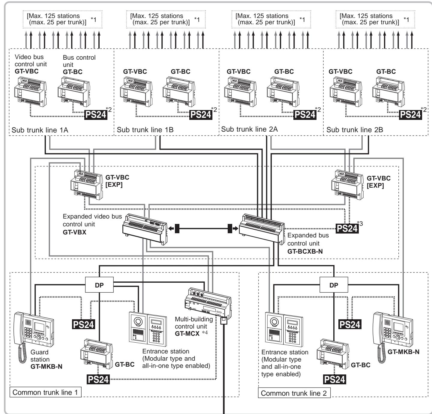
\*4: The multi-building control unit GT-MCX must be connected to common trunk line 1.
