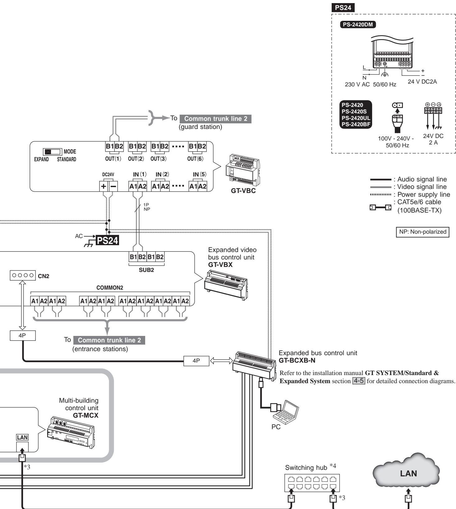
\*3: Do not route a CAT5e/6 cable outdoors from a multi-building control unit directly. When routing a CAT5e/6 cable outdoors from a switching hub, use a model that supports outdoor wiring.
