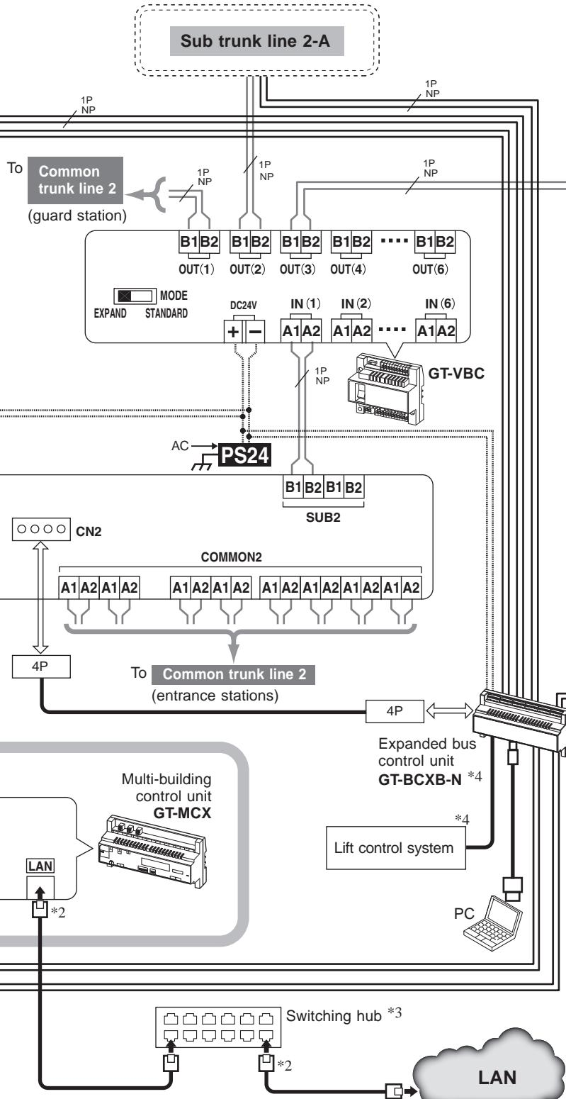
\*2: NOTE: Do not route a CAT5e/6 cable outdoors from a multi-building control unit directly. When routing a CAT5e/6 cable outdoors from a switching hub, use a model that supports outdoor wiring.
