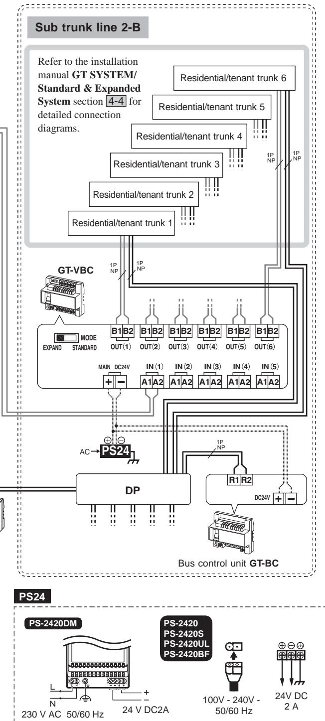
\*4: Refer to the installation manual **GT SYSTEM/Standard & Expanded System** sections [4-5] to [4-6] for details about the lift control system.
