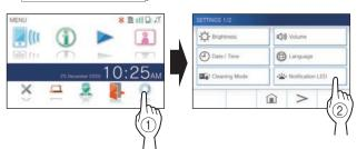
2 Tap ON to turn notification LED on, or OFF to turn the notification LED off.
