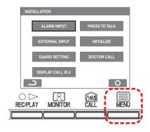
**3** To finish changing settings, press the [○ OFF] button to return to the standby mode. In other cases, set by pressing the [■ MENU] button. Press the [○▷ REC/PLAY] button to cancel the settings and return to the previous screen.
