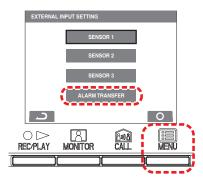
**6** Select from "ENABLE/DISABLE" in the "SECURITY ALARM TRANSFER" screen. Press the [■ MENU] button to complete the settings.
