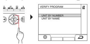
5 Display the unit by using the 10 key, then press (a) or (b).
