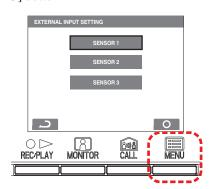
3 Select from "DISABLE/UTILITY/SECURITY" in each screen from "SENSOR1 SETTING" to "SENSOR3 SETTING" and then press the [■ MENU] button.
