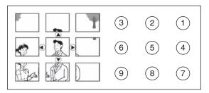
**Setting method**: Select the desired position number ① to ⑨ by using the 10-key.
