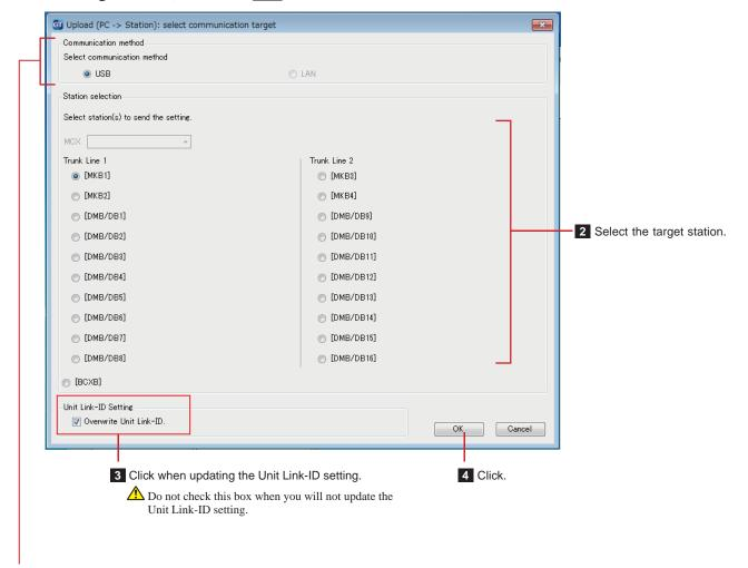
1 Select the communication method with the target station.
