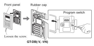
The IN USE LED will flash, and then change to being lit to show that the unit has entered into the programming mode.
