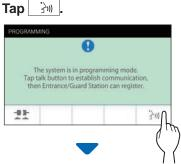
The corresponding communication channel will be established.
