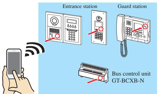
The manager or admin code is read by the target station, and the setting file is uploaded.
