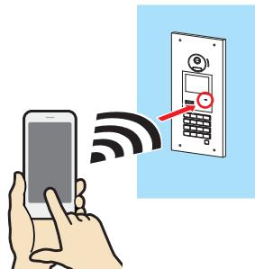
The passcode or NFC card ID is read by the target station, and the picture is uploaded.
