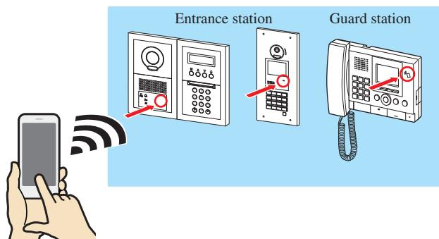
The NFC card ID is read by the target station, and the setting file is downloaded.
