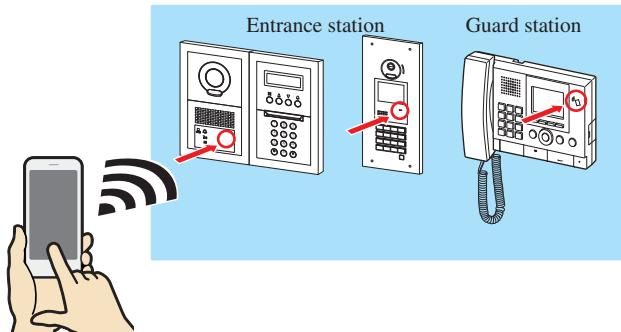
The NFC card ID is read by the target station, and the setting file is uploaded.
