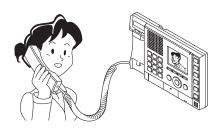
When you have finished the communication, put the handset on the hook. Communication will end.
