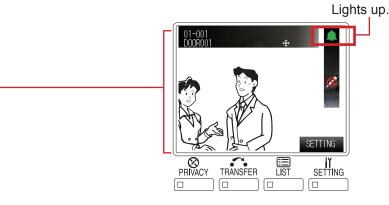
The station no., station name and video image at the calling station (following the symbol image) are displayed. (When called from a remote site, the site no., site name and video image at the calling station (following the symbol image) are displayed. The station name will not be displayed.)
